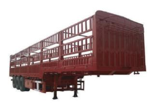
POULTRY CARRING TRUCKS (BOX TYPE STRUCTURE OF HORIZONTAL ROWS ALONG THE WIDTH)
