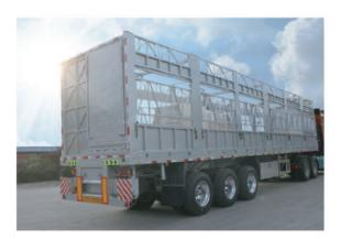
LIVE STOCK CARRIER (DIFFERENT KIND OF ARRANGEMENTS SHOULD BE MADE DEPENDING UPON PAYLOAD)
